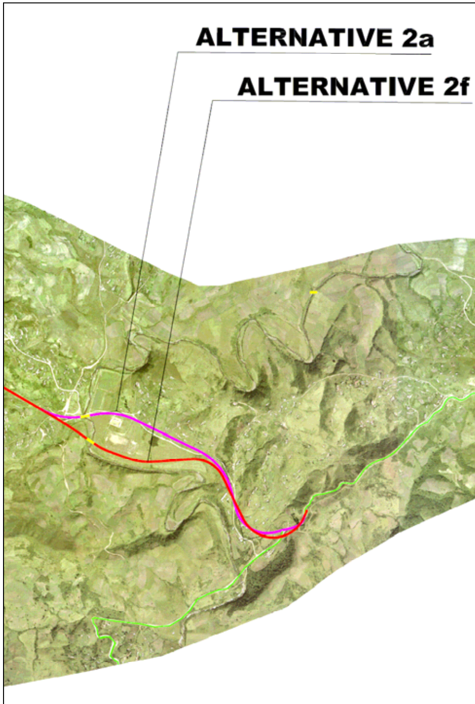
FIG 6.2 Alternative Alignments: Vicinity of Ntafufu Village and River (Alternative 2f is the SANRAL preferred route (in red))
