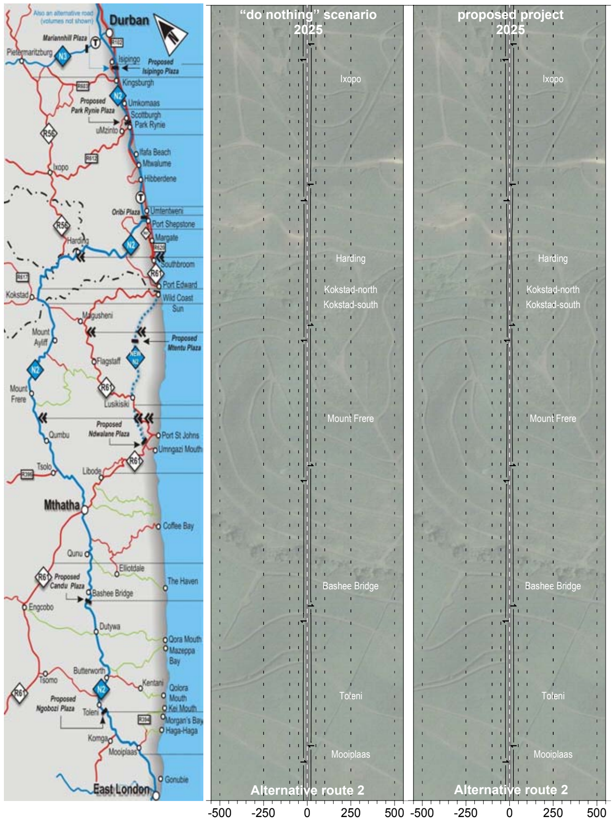
Figure A6.26: Comparison of modelled ambient concentrations of CO for the "do nothing" scenario ("existing routes"/without new roads and new tolls) against concentrations for the scenario "with new roads and new tolls" (the proposed project) in year 2025 for the existing route (Alternative) 2 (R56 and existing N2). Red lines indicate predicted exceedances of the SANS limit value ( 30 \text{ mg/m}^3 )
