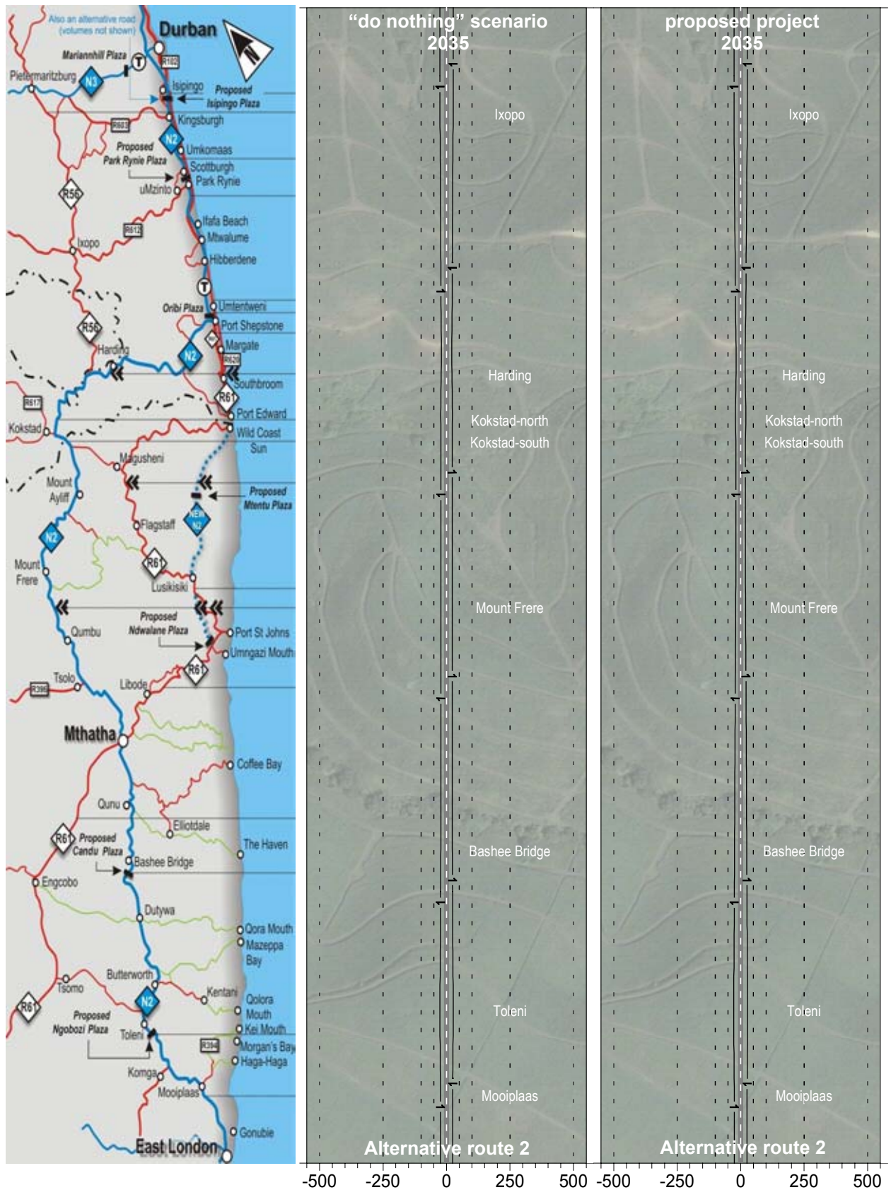
Figure A6.35: Comparison of modelled ambient concentrations of CO for the "do nothing" scenario ("existing routes"/without new roads and new tolls) against concentrations for the scenario "with new roads and new tolls" (the proposed project) in year 2035 for the existing route (Alternative) 2 (R56 and existing N2). Red lines indicate predicted exceedances of the SANS limit value (30 mg/m 3 )
