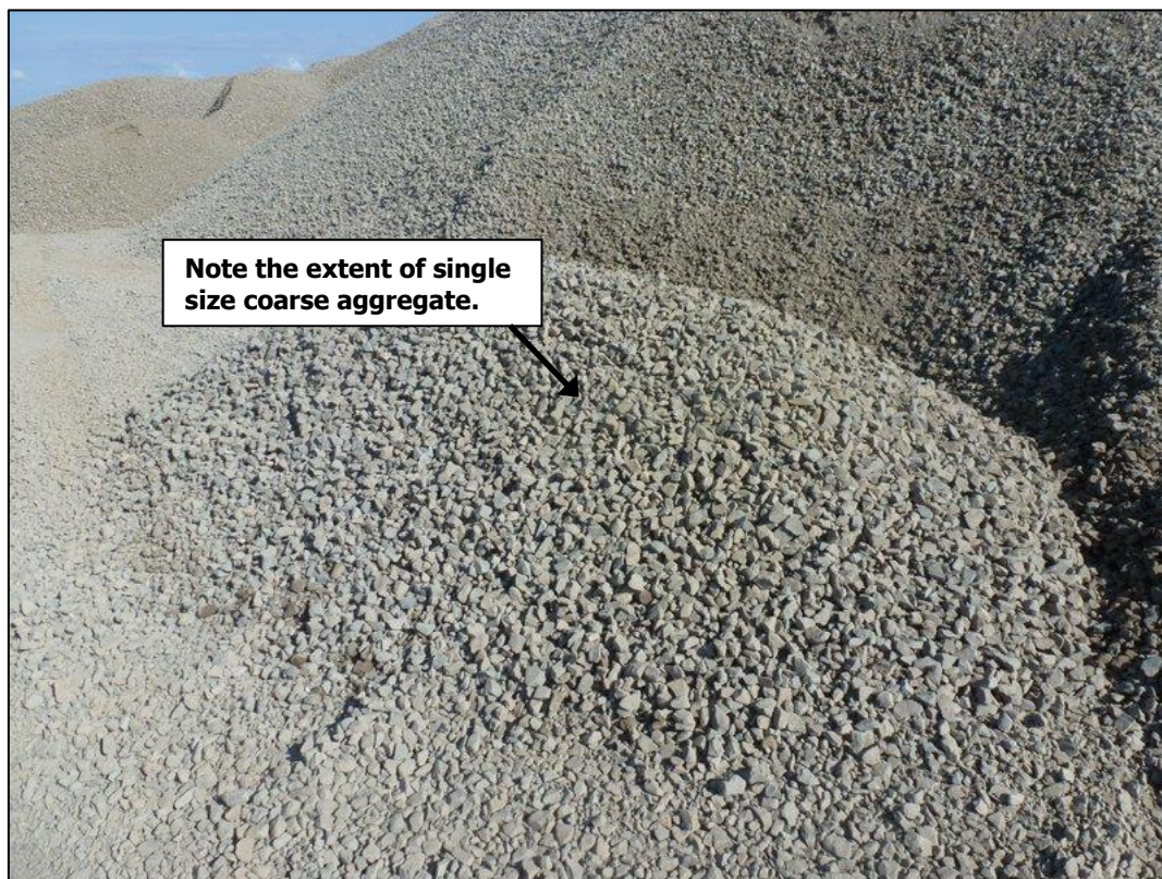
Figure 76. Segregated Material in Stockpile
