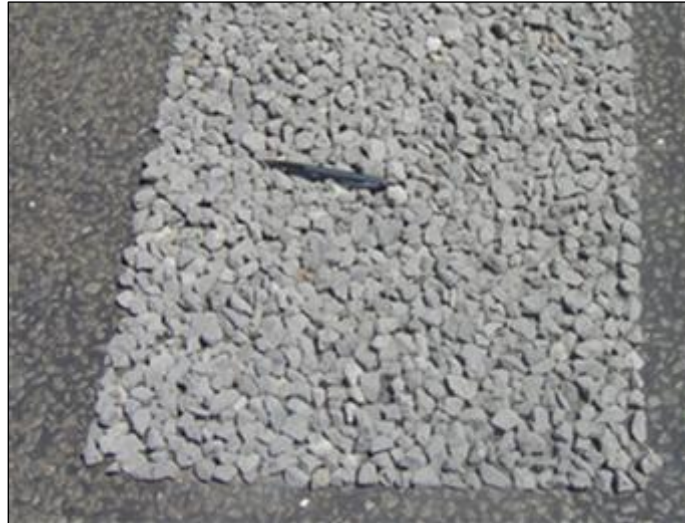
Figure 91. Target Matrix by Hand Packing
