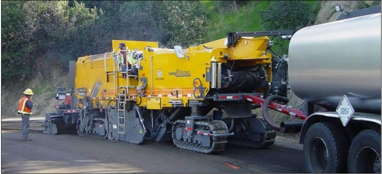
Figure 45. Example of a Track Mounted Recycler
