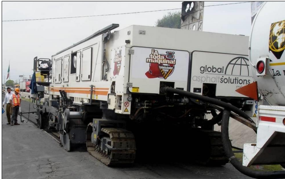
Figure 47. Recycling Machine Fitted with On-Board Mixing Unit
