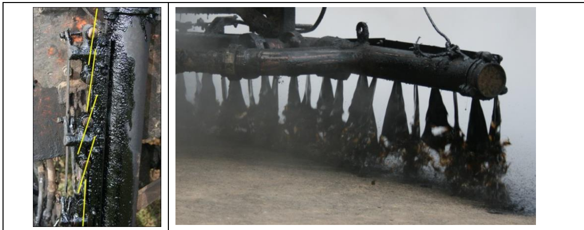
Figure 85. Flair Interference Due to Wrong Angle Settings
