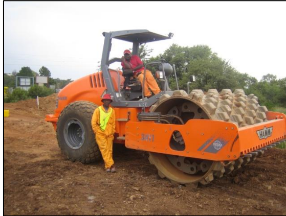
Figure 61. Single Wheel Padfoot Roller
