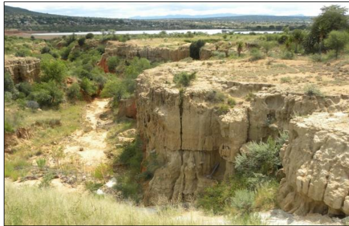
Figure 67. Erosion of Dispersive Soil Type
