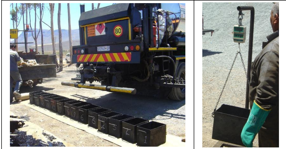
Figure 84. Transverse Distribution Bakkie/Bucket Test
