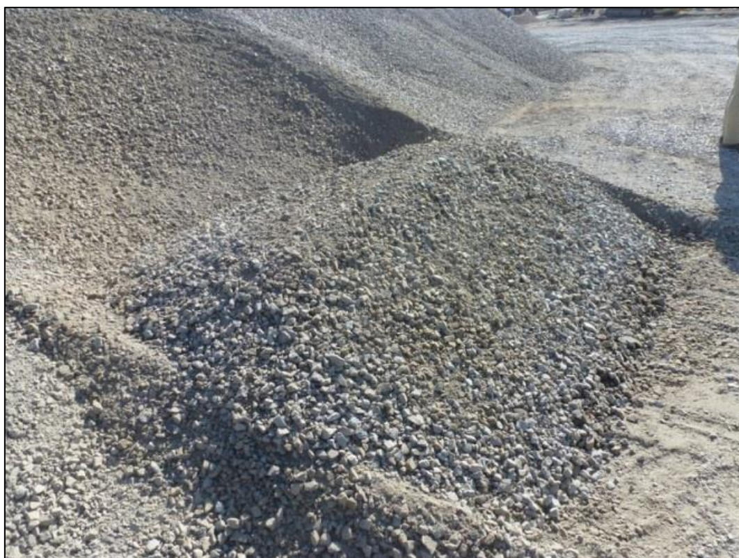
Figure 77. Suitable Stockpile with No Sign of Segregation
