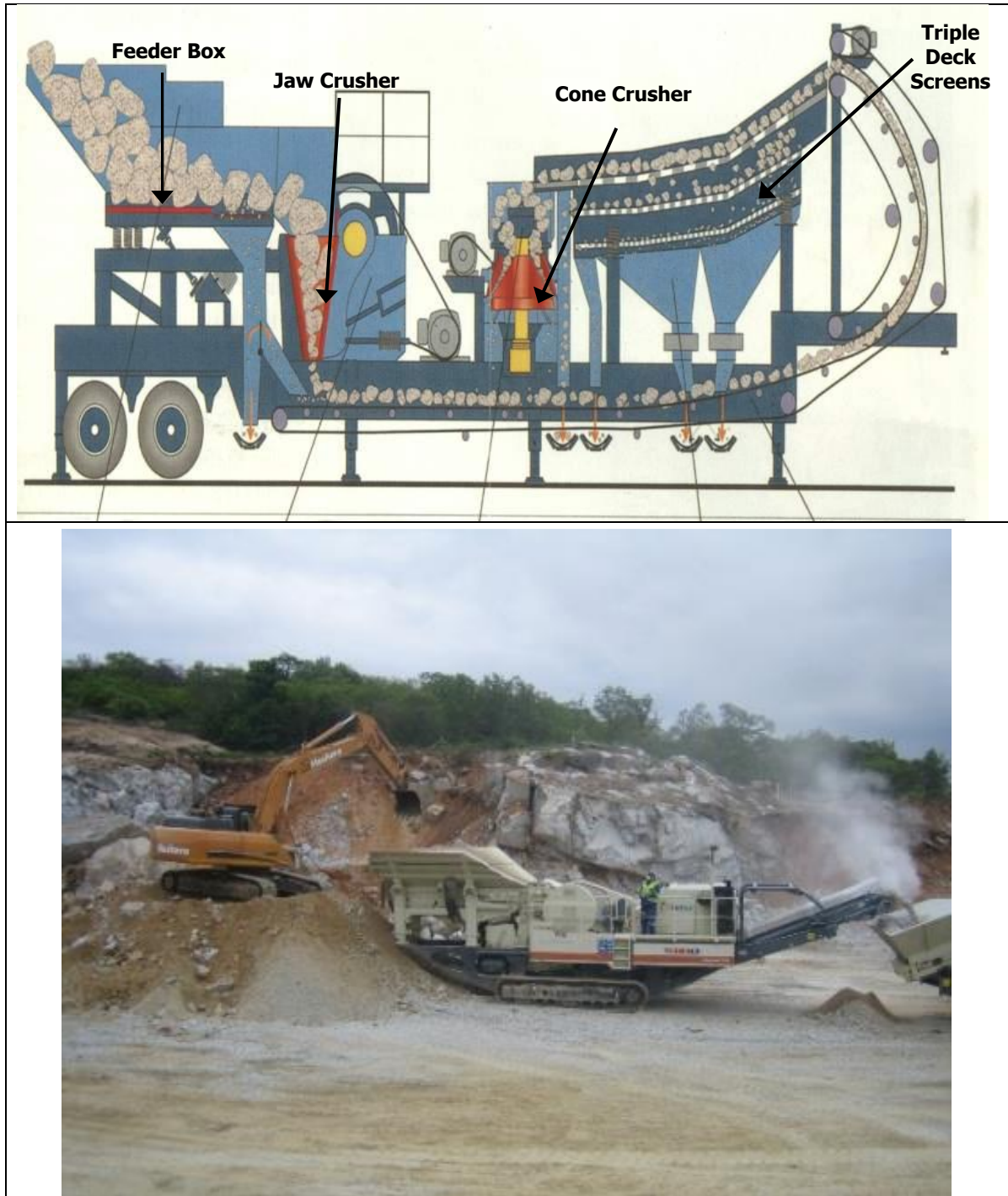
Figure 8. Mobile Jaw & Cone Crusher with Screens
