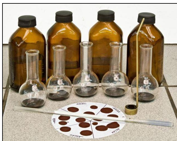
Figure 16. N-Heptane/Xylene Spot Test
