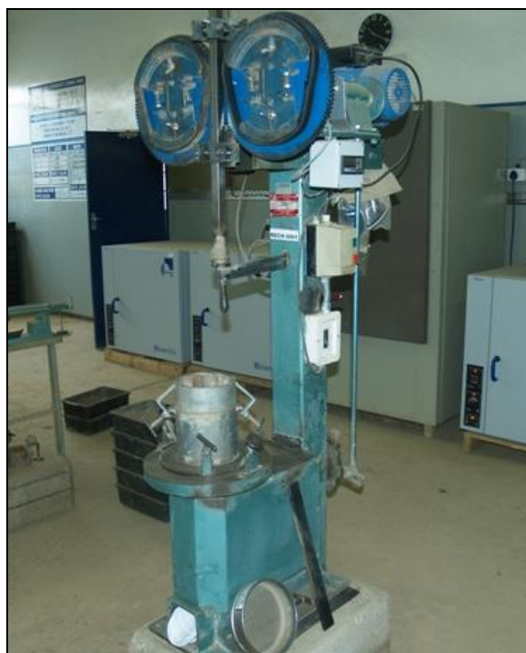
Figure 6. Soil Compaction Equipment (with protective coverings removed for illustration)
