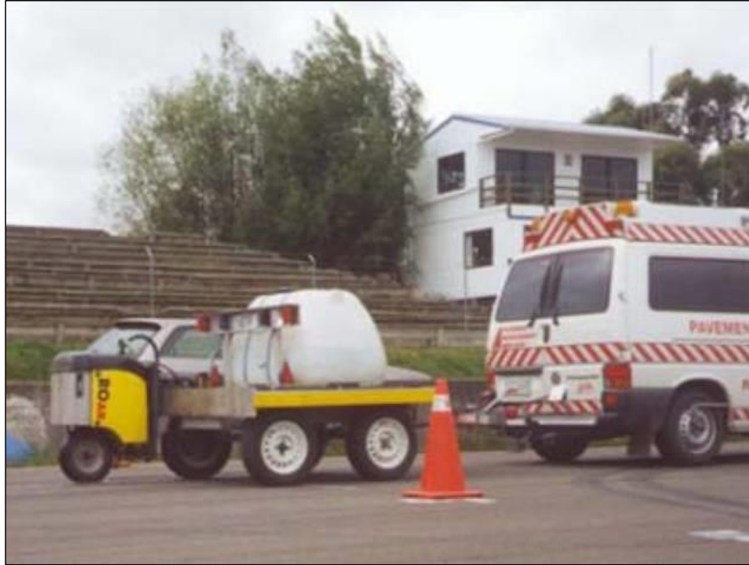
Figure 35. Norsemeter to Measure Micro Texture
