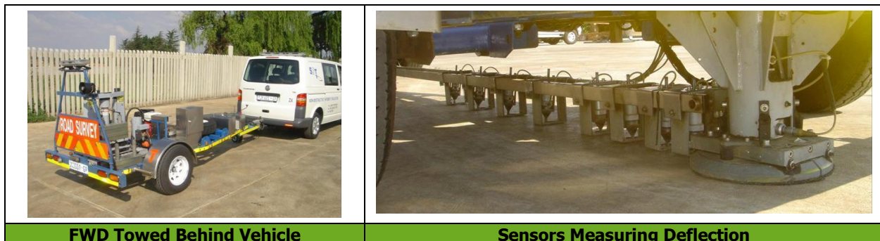
Figure 39. Falling Weight Deflectometer (FWD) for Measuring Deflection
